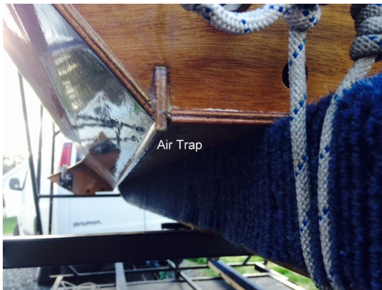
Figure 9. The rear view of a typical left airtrap. This one is about \frac{1}{4} inch deep at the transom.
