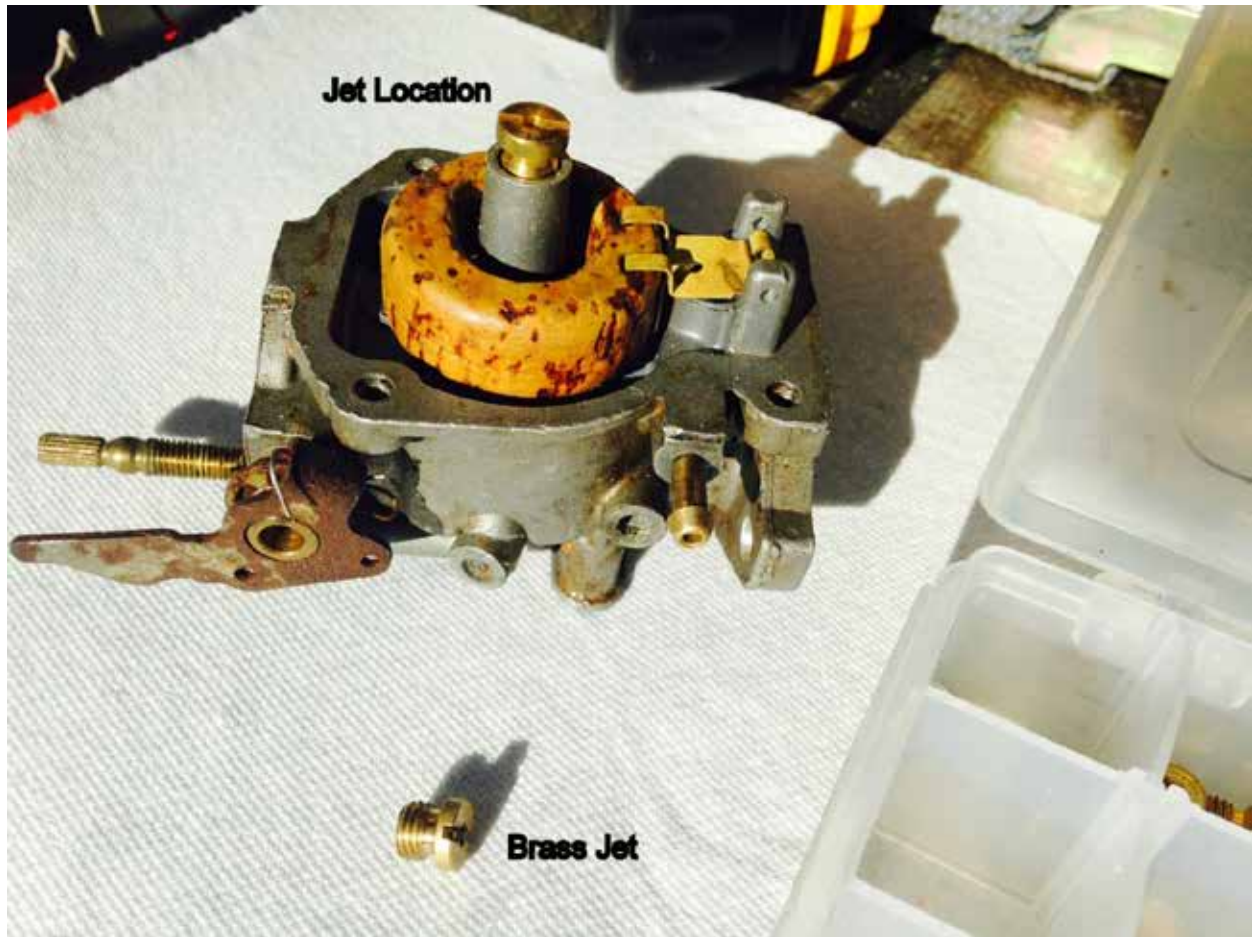
Figure 12. OMC A carb with float bowl removed. The brass jet is located on the top and another jet is shown on the workbench.
