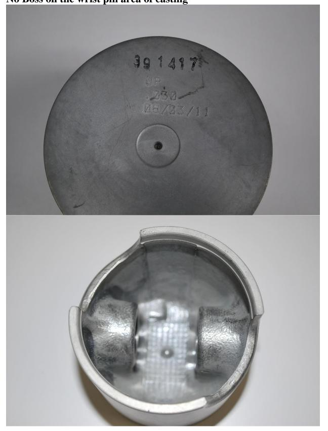
OEM Piston - PN 391417 – Distinctive OMC lettering on the top. No Boss on the wrist pin area of casting
