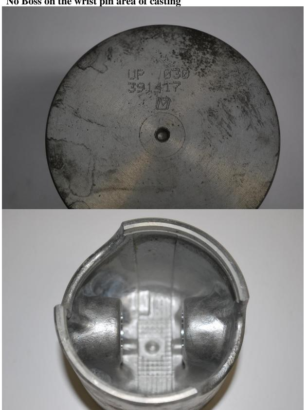
OEM Piston - PN 5006665 – Distinctive OMC/BRP lettering on the top. No Boss on the wrist pin area of casting
