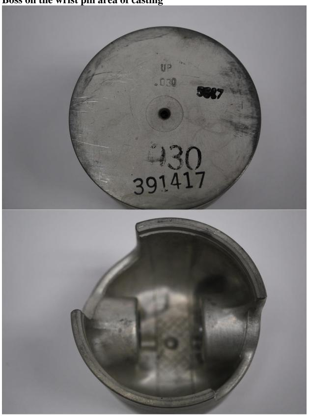
Pro Marine Piston – Looks identical to the OEM Piston – Notable differences is the stamped lettering on the top of the piston (Extra dimensional number's and the fact that the sizing runs horizontal to the "UP" lettering). Secondly note casting Boss on the on the wrist pin
