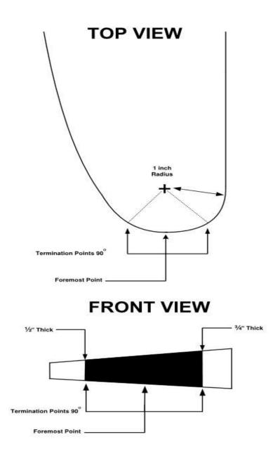
A. On boats equipped with breakaway pickleforks and breakaway cockpit noses that meet a laminate thickness of no more than 1/16" or 1.5 mm, the breakaway part must contain no material other than the outer shell. The boat must also provide a way for inspection. The collapsible section must be a minimum of 3" and have a bulkhead at the start of the non-breakaway part of the sponson.
