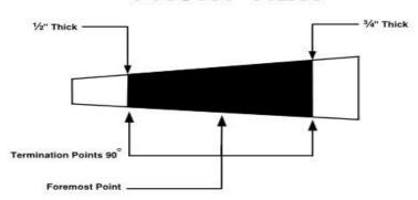
A. On boats equipped with breakaway pickleforks and breakaway cockpit noses that meet a laminate thickness of no more than 1/16" or 1.5 mm, the breakaway part must contain no material other than the outer shell. The boat must also provide a way for inspection. The collapsible section must be a minimum of 3" and have a bulkhead at the start of the non-breakaway part of the sponson.
