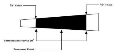
A. On boats equipped with breakaway pickleforks and breakaway cockpit noses that meet a laminate thickness of no more than 1/16" or 1.5 mm, the breakaway part must contain no material other than the outer shell. The boat must also provide a way for inspection. The collapsible section must be a minimum of 3" and have a bulkhead at the start of the non-breakaway part of the sponson.
