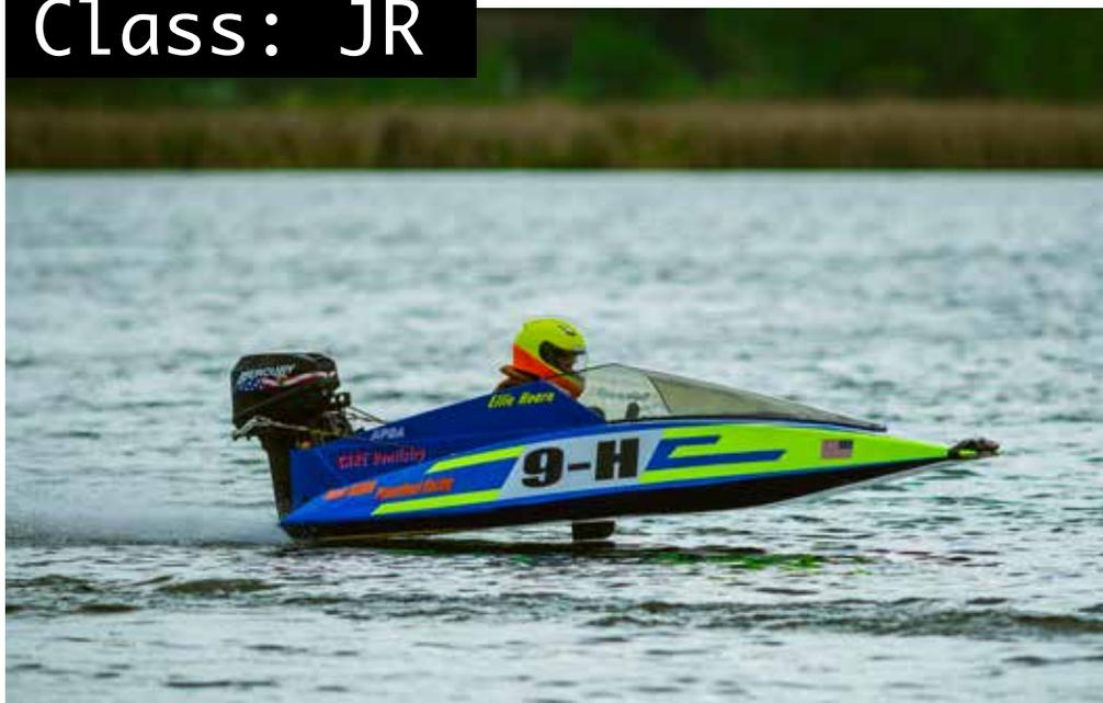
Junior Runabouts are made to slice through the water. Kids can drive J Runabouts in both circle races (around an oval track marked by buoys) and in marathons, which can be many laps of an oval course or a point-to-point long-distance race. The driver kneels in the cockpit, steering with the right hand and squeezing the throttle with the left. A runabout can handle rough water if the driver has the skill to handle it.
