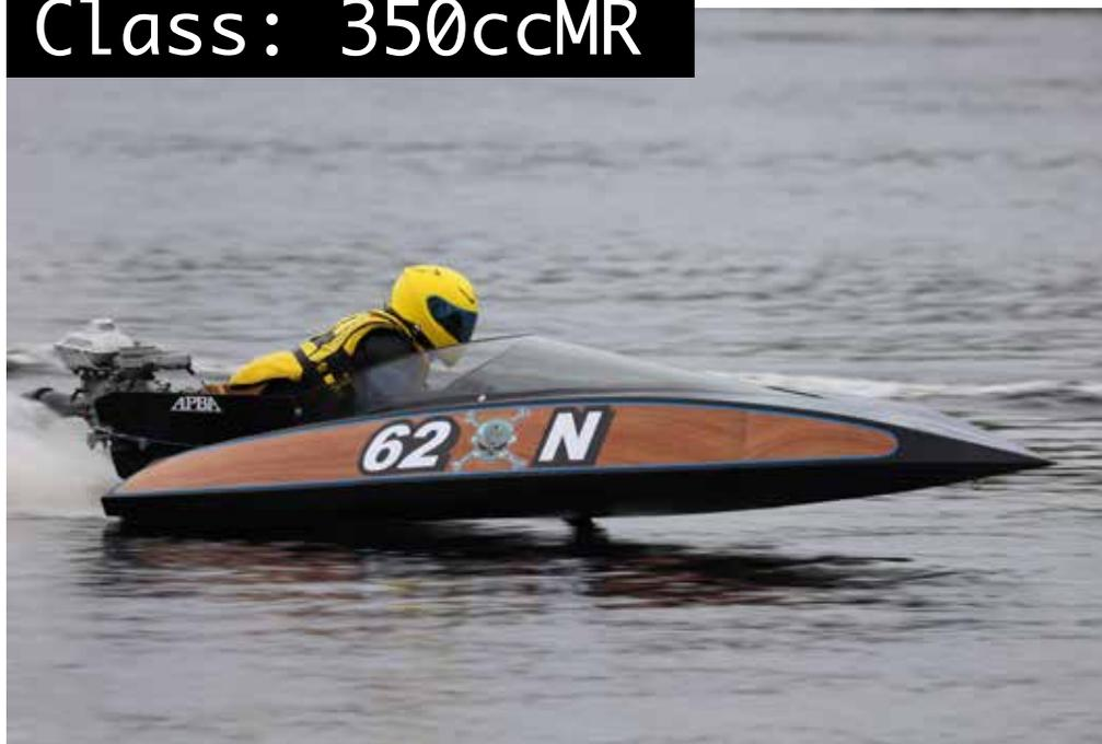
The 350cc class is another class that challenges the technical savvy racer. Legal engines include modified Yamato 80 engines with expansion chamber exhaust, or a stock Mercury 25xs. Many modified racers claim that this is the greatest ride with a high horsepower to weight ratio.
