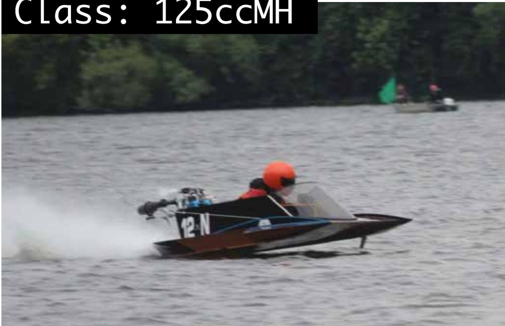
The 125cc Modified Hydroplane (125ccMH) class is in its third year of existence in APBA racing. Go-kart tested and developed, PRD Fireball engines power these small hydroplanes as they fly across the water.
