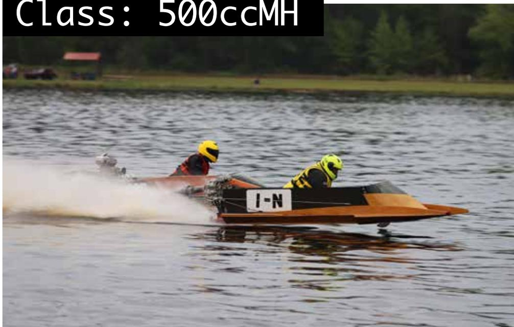
The 500cc class is an exciting class offering competitors the option to run highly modified Mercury Mark 30H engines, or modified Yamato 102 or 302 engines with expansion chamber exhaust. The combination of these two available engines provides exciting competition, with the 4 cylinder Mercury's competing against the 2 cylinder Yamatos.
