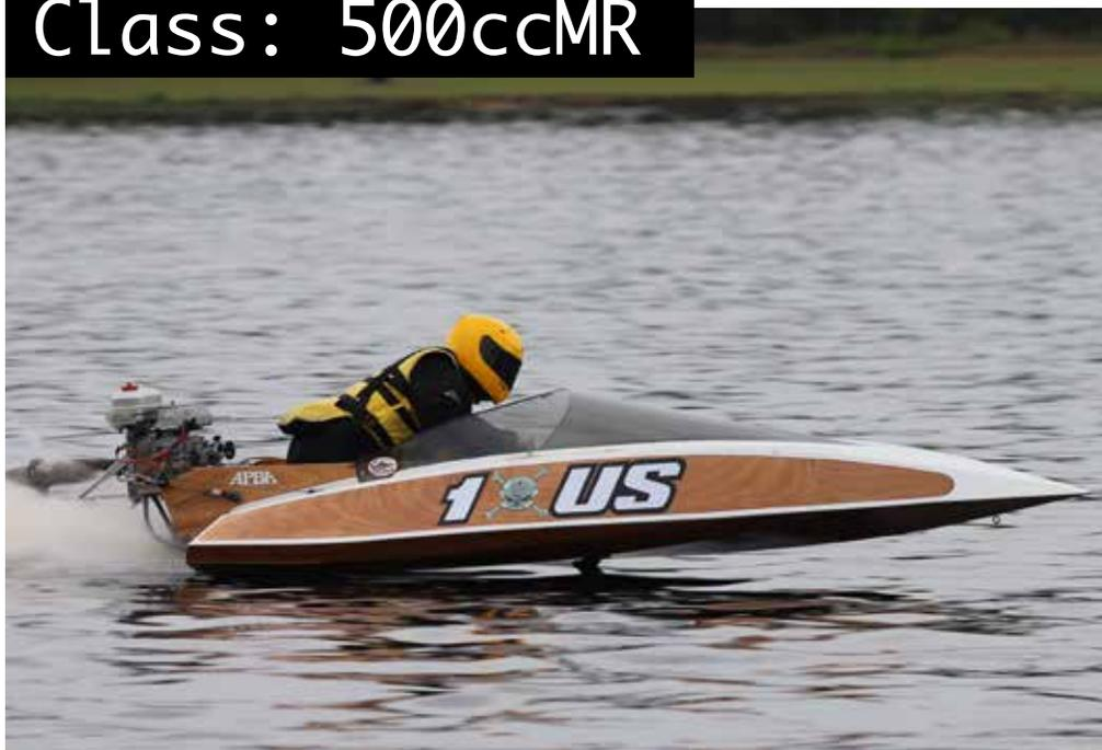
The 500ccMR class is an exciting class offering competitors the option to run highly modified Mercury Mark 30H engines, or modified Yamato 102 or 302 engines with expansion chamber exhaust. The combination of these two available engines provides exciting competition, with the 4 cylinder Mercury's competing against the 2 cylinder Yamatos.
