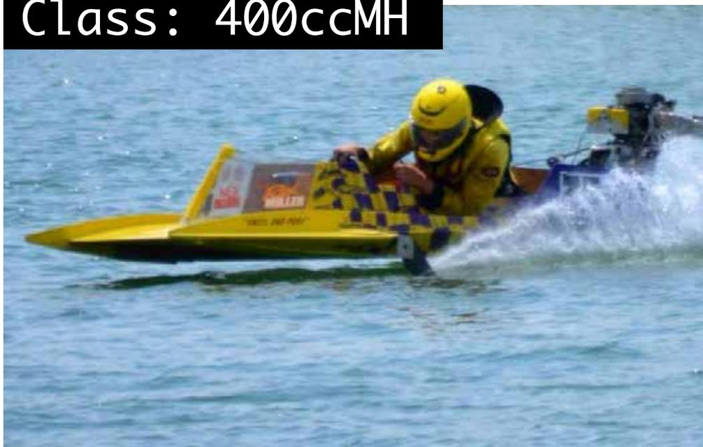
Using highly modified Mercury and OMC 2 cylinder engines, this class produces a roar like no other using its single megaphone exhaust, producing speeds in excess of 65 MPH.
