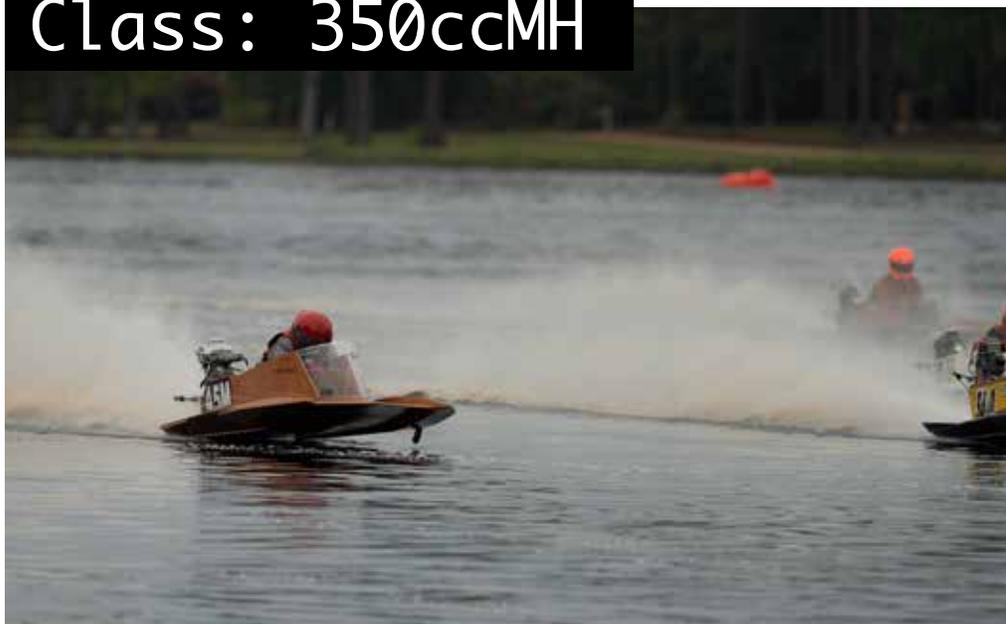
The 350cc class is another class that challenges the technical savvy racer. Legal engines include modified Yamato 80 engines with expansion chamber exhaust, or a stock Mercury 25xs. Many modified races claim that this is the greatest ride with a high horsepower to weight ratio.
