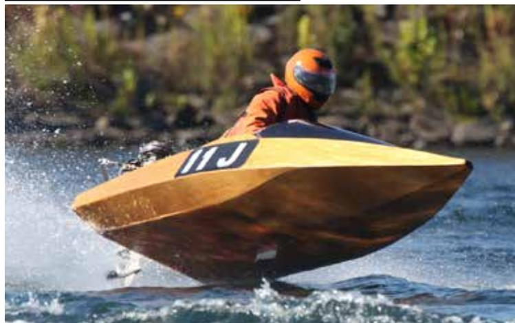
Stock and Mod Outboard runabouts are a distant cousin to the average pleasure boat. Similar to the family runabout in that it is a displacement craft, the runabout is slower than the hydroplane. Without front sponsons to help trap air and stabilize the boat, the runabout is more affected by the water conditions and drivers must continually work the boat in order to keep it level. Physically demanding, the runabout is similar to riding a motorcross dirt bike.
