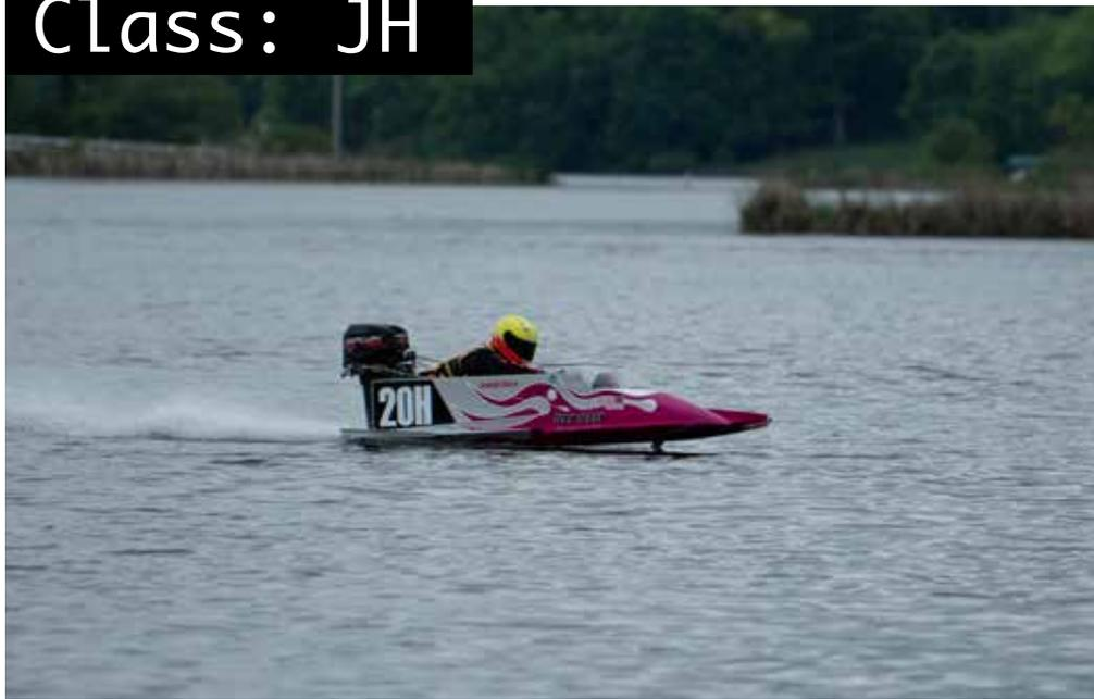
Junior Class Hydroplanes are made to skim across the water, with only the propeller and sponsons (the projecting parts on either side of the hull) touching the surface. The trick is to allow just enough air to rush underneath the boat, giving it the lift that allows J Hydros to hit speeds of 45 MPH or more. Drivers steer with the right hand and squeeze the throttle with the left, kneeling in the cockpit and staying low to minimize drag.
