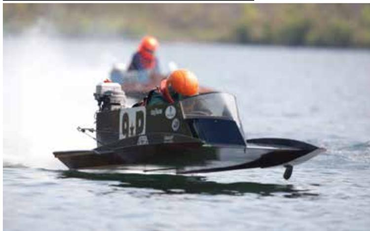
Modern hydros are constructed with a three point design, meaning three points of contact with the water. Those points are the two front sponsons and the bottom of the boat near the transom. Hydros are designed to trap air underneath the boat, causing the sponsons to lift out of the water when the boat is traveling in a straight line. The boat is designed to ride on this cushion of air and truly skim across the top of the water.
