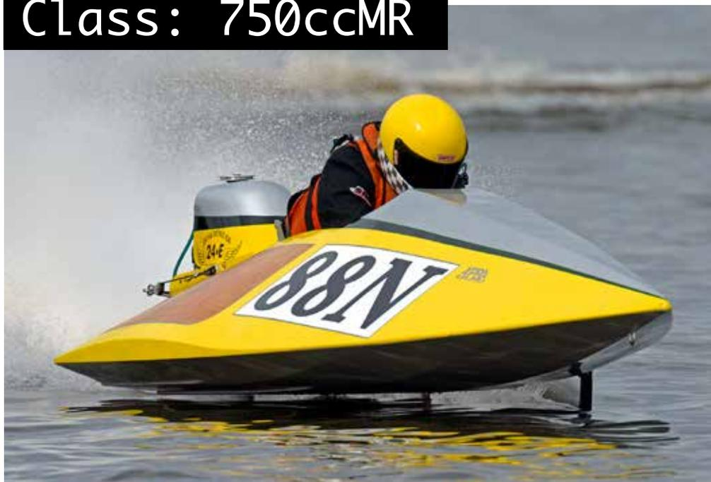
The 750cc Mod R class is comprised of the toughest Modified competitors on the water. Highly modified Mercury 4 cylinder engines with mega-phone exhaust power these boats well past the 85 MPH mark, and are not for the faint of heart.
