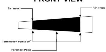
A. On boats equipped with breakaway pickleforks and breakaway cockpit noses that meet a laminate thickness of no more than 1/16" or 1.5 mm, the breakaway part must contain no material other than the outer shell. The boat must also provide a way for inspection. The collapsible section must be a minimum of 3" and have a bulkhead at the start of the non-breakaway part of the sponson.
