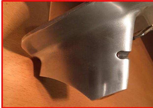
This guide is a supplement to the Stock Outboard Technical Manual. This is a suggested guide on how to enhance the water inlet hole of the Yamato engines.
