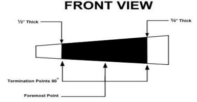
A. On boats equipped with breakaway pickleforks and breakaway cockpit noses that meet a laminate thickness of no more than 1/16" or 1.5 mm, the breakaway part must contain no material other than the outer shell. The boat must also provide a way for inspection. The collapsible section must be a minimum of 3" and have a bulkhead at the start of the non-breakaway part of the sponson.
