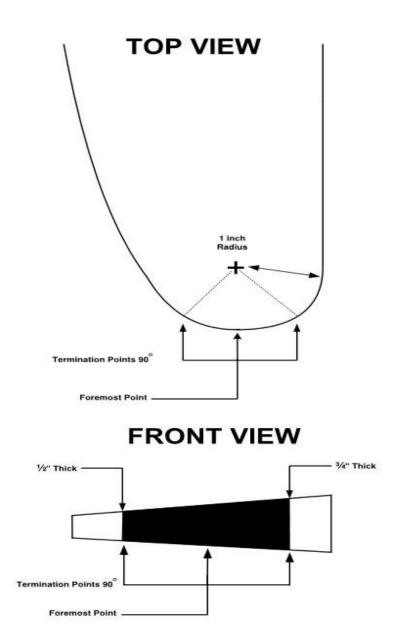
A. On boats equipped with breakaway pickleforks and breakaway cockpit noses that meet a laminate thickness of no more than 1/16" or 1.5 mm, the breakaway part must contain no material other than the outer shell. The boat must also provide a way for inspection. The collapsible section must be a minimum of 3" and have a bulkhead at the start of the non-breakaway part of the sponson.
