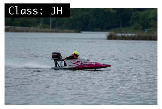
Junior Class Hydroplanes are made to skim across the water, with only the propeller and sponsons (the projecting parts on either side of the hull) touching the surface. The trick is to allow just enough air to rush underneath the boat, giving it the lift that allows J Hydros to hit speeds of 45 MPH or more. Drivers steer with the right hand and squeeze the throttle with the left, kneeling in the cockpit and staying low to minimize drag.
