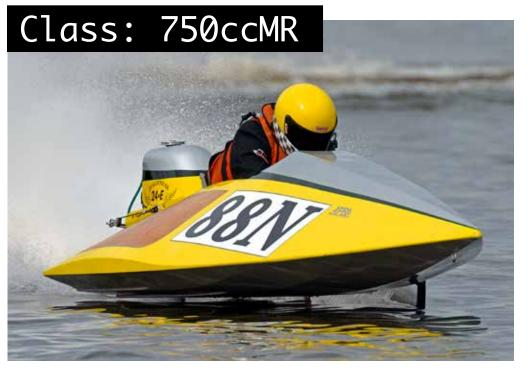
The 750cc Mod R class is comprised of the toughest Modified competitors on the water. Highly modified Mercury 4 cylinder engines with megaphone exhaust power these boats well past the 85 MPH mark, and are not for the faint of heart.
