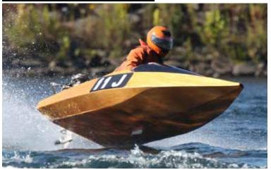
Stock and Mod Outboard runabouts are a distant cousin to the average pleasure boat. Similar to the family runabout in that it is a displacement craft, the runabout is slower than the hydroplane. Without front sponsons to help trap air and stabalize the boat, the runabout is more affected by the water conditions and drivers must continually work the boat in order to keep it level. Physically demanding, the runabout is similar to riding a motorcross dirt bike.
