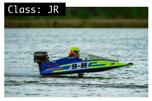
Junior Runabouts are made to slice through the water. Kids can drive J Runabouts in both circle races (around an oval track marked by buoys) and in marathons, which can be many laps of an oval course or a point-to-point long-distance race. The driver kneels in the cockpit, steering with the right hand and squeezing the throttle with the left. A runabout can handle rough water if the driver has the skill to handle it.
