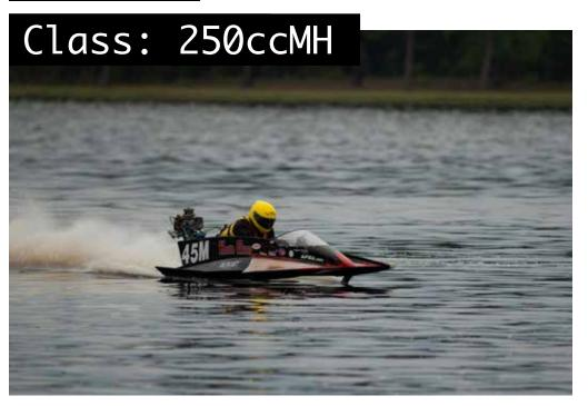
250cc Modified Hydro (250ccMH), Also known as "A Mod" or AMH Displacement: Starting at 12.5 cubic inches up to 15 cubic inches. Mark20H (20 cubic inch Mercury engine with 1987 Stock Outboard specifications).
