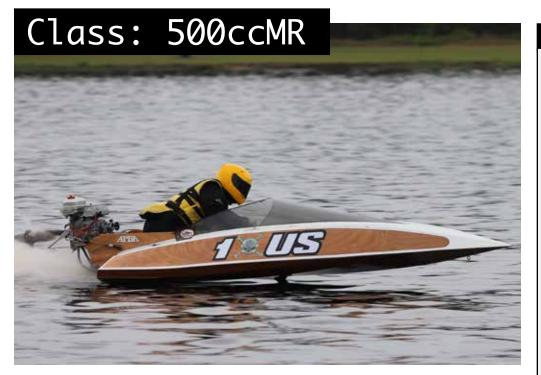
The 500ccMR class is an exciting class offering competitors the option to run highly modified Mercury Mark 30H engines, or modified Yamato 102 or 302 engines with expansion chamber exhaust. The combination of these two available engines provides exciting competition, with the 4 cylinder Mercury's competing against the 2 cylinder Yamatos.
