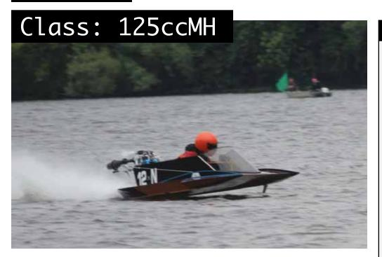
The 125cc Modified Hydroplane (125ccMH) class is in its third year of existence in APBA racing. Go-kart tested and developed, PRD Fireball engines power these small hydroplanes as they fly across the water.
