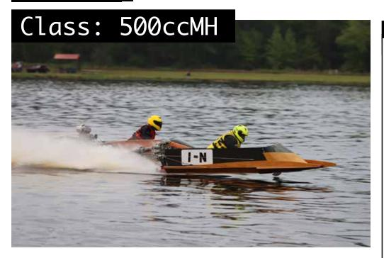
The 500cc class is an exciting class offering competitors the option to run highly modified Mercury Mark 30H engines, or modified Yamato 102 or 302 engines with expansion chamber exhaust. The combination of these two available engines provides exciting competition, with the 4 cylinder Mercury's competing against the 2 cylinder Yamatos.
