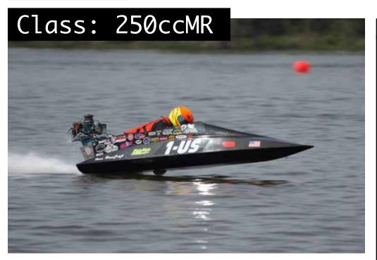
250cc Modified Runabout (250ccMR), Also known as "A Mod" or AMR Displacement: Starting at 12.5 cubic inches up to 15 cubic inches. Mark20H (20 cubic inch Mercury engine with 1987 Stock Outboard specifications)..
