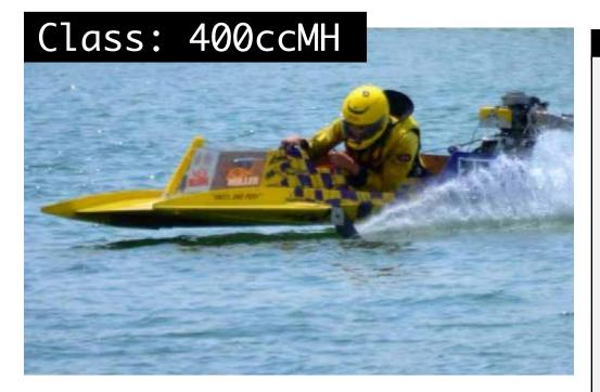
Using highly modified Mercury and OMC 2 cylinder engines, this class produces a roar like no other using its single megaphone exhaust, producing speeds in excess of 65 MPH.
